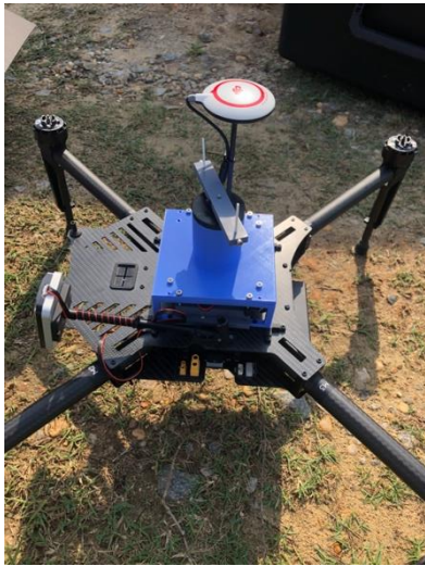
Figure 4: Spore-trapping drone to sample large-acreage fields for Pseudoperonospora cubensis sporangia.
