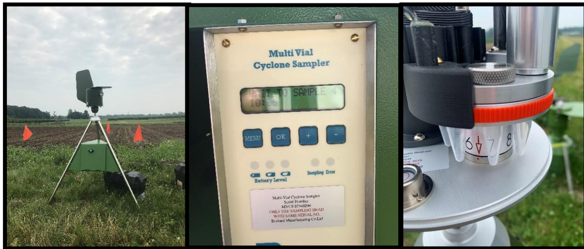
Figure 2. Cyclone spore traps tested in Michigan have rotating vials instead of a sticky tape that could lead to quicker processing of air samples to return results to growers quickly.
