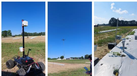
Figure 5. Spore trap in rover, hanging from UAV, with a wind sensor.
